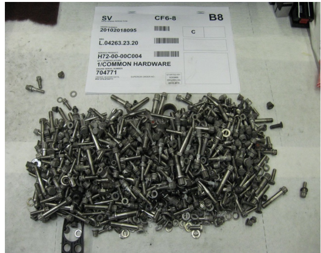
Figure 1: Fasteners that were taken from part of airplane engine and must be classified during an overhaul process.
