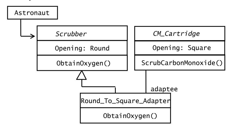
Using a carbon monoxide scrubber (round opening) in the lunar module with square cartridges from the command module (square opening)
