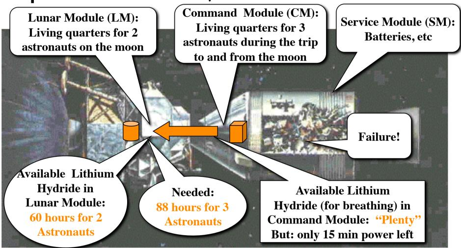
The LM was designed for 60 hours for 2 astronauts staying 2 days on the moon Redesign challenge: Can the LM be used for 12 man-days (2 1/2 days until reentry into Earth)?
