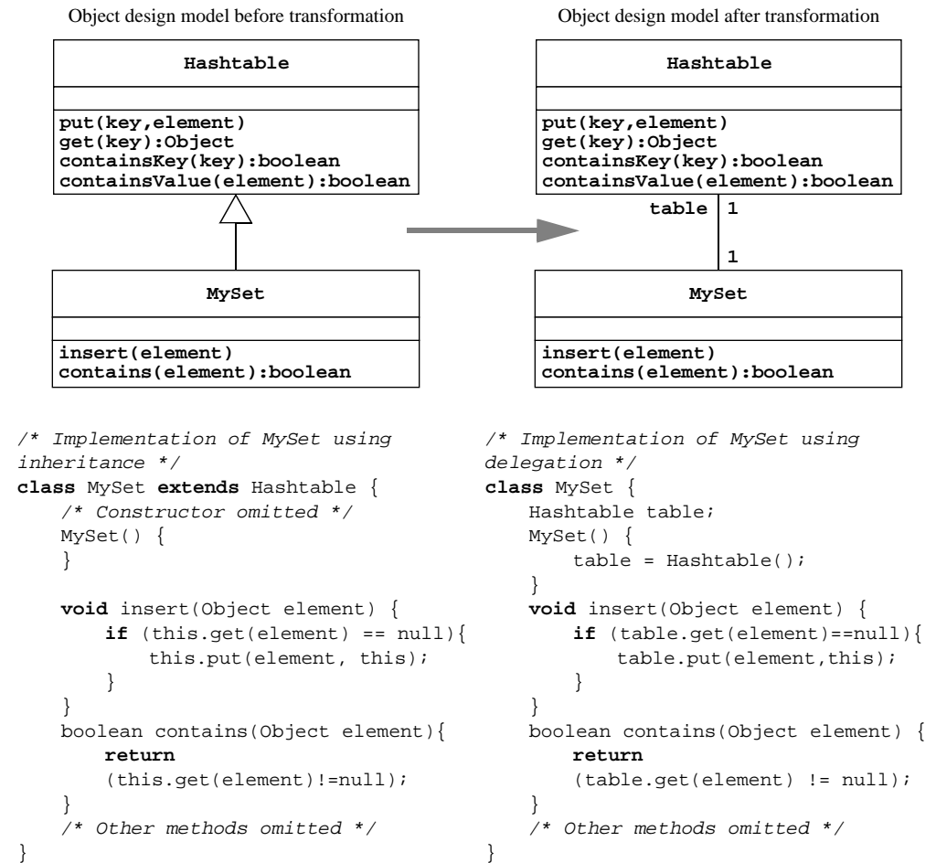
Figure 7-29 An example of implementation inheritance. The left column depicts a questionable implementation of MySet using implementation inheritance. The right column depicts an improved implementation using delegation. (UML class diagram and Java).
